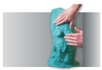
Smoothing the last layer. After finishing the filler layers, it can be smoothed with a mild soap solution to get a homogeneous surface.
