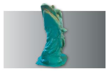
The second layer is also applied thinly after the first layer has gelled. The silicone is now already thickened with Thixo Additive RTV-3011, but still flowable.
