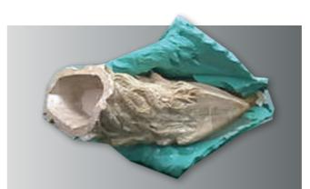
The silicone negative is cut open and removed from the master model. Then the mould is reassembled in reverse order.
