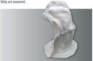
After coating the separation area with Honey Wax, the second half is laminated.
