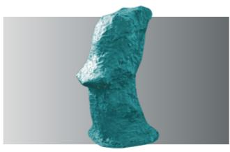
The finished silicone negative before building the ebacryl supporting mould.
