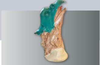
The first layer of silicone SILASTIC™ RTV-4250 S is applied thinly with a brush. The layer should be blister-free.
